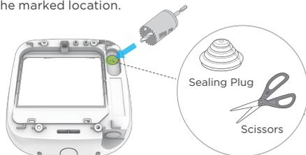
**Note:** If you want to use the M20 SWA copper gland for cable feeding. Please use the M25 to M20 reducer in the accessories instead of the sealing plug, then use a spanner to secure it.
