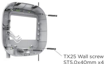
**Note:** Suggested installation torque 3Nm+/-10% (different materials of walls have different torques), to avoid over-tightening and cracking the casing.
