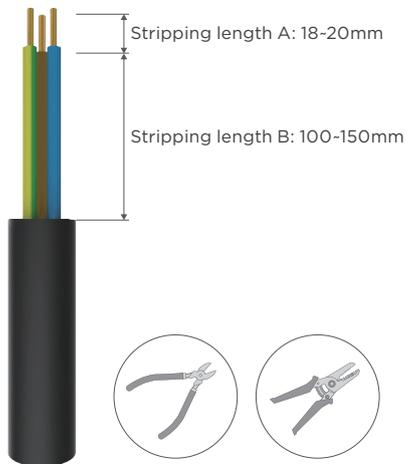
Stripping length B depends on the cable entry you choose. The above diagram shows a range recommended by the manufacturer, choose the optimum length according to the individual requirements of your set up.
